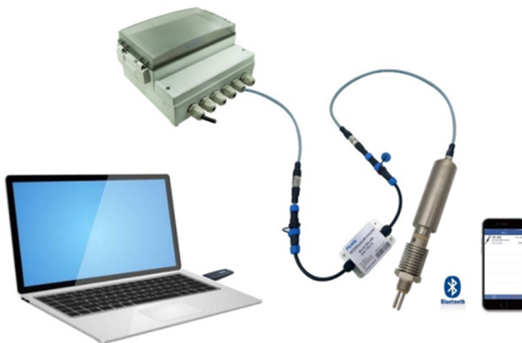
Figure 9. Bluetooth connection to CR-301 sensor
